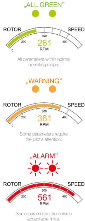
Fig. 7. The idea of flight parameter status information
