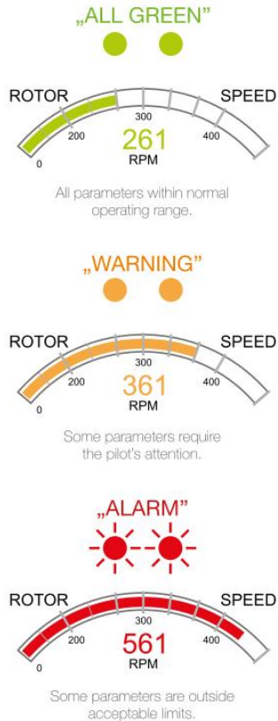
Fig. 7. The idea of flight parameter status information
