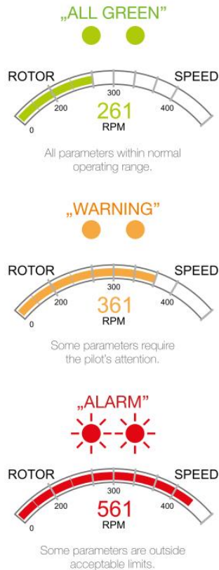
Fig. 7. The idea of flight parameter status information
