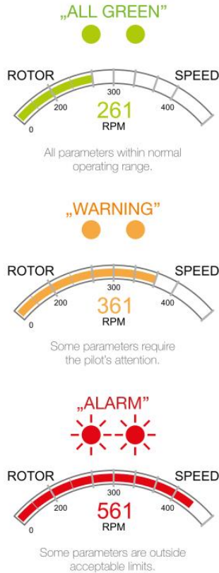
Fig. 7. The idea of flight parameter status information
